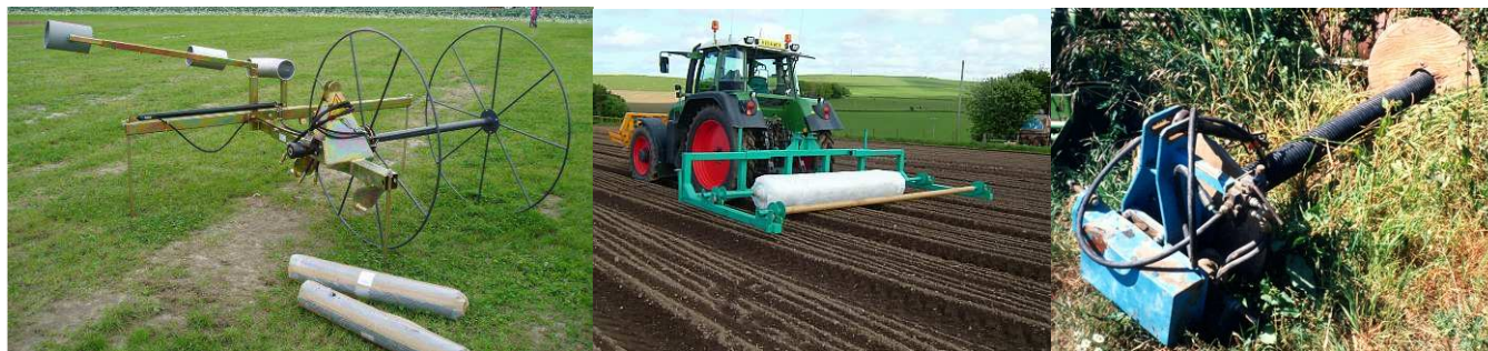
Figure 8. Three examples of floating crop cover handling systems all using removable bobbins (center photo courtesy www.wondermesh.co.uk ).
