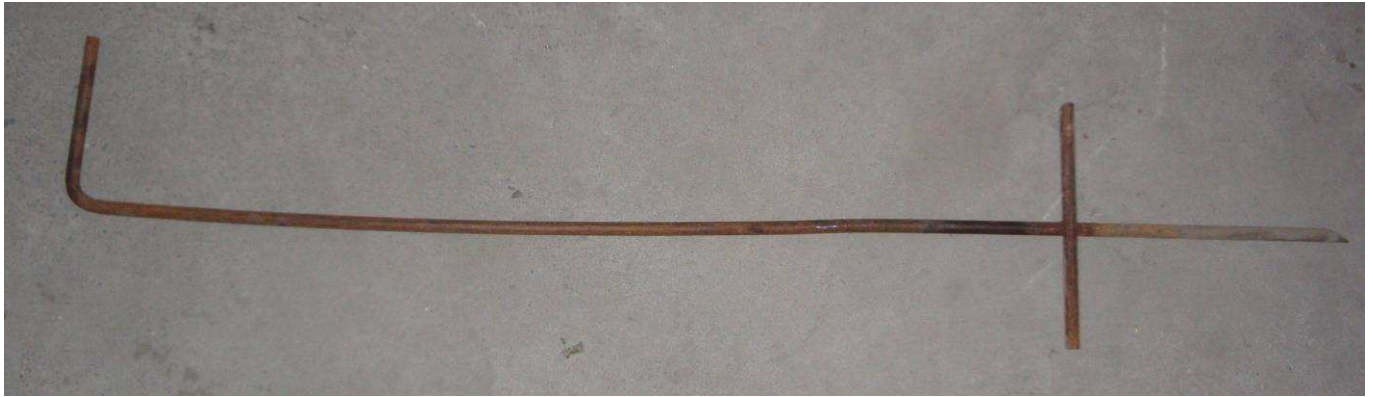
Figure 9. Custom steel stake for holding down floating crop covers.
