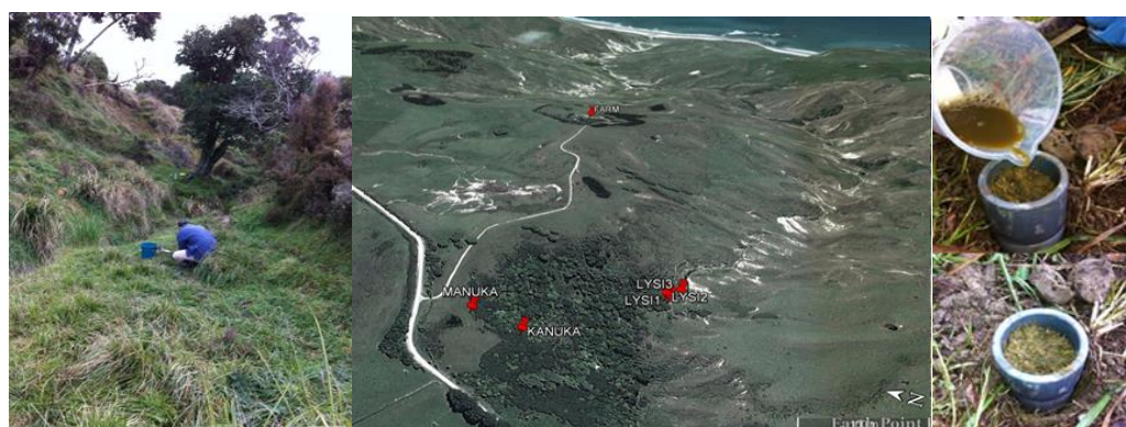
Figure 15: Taiporutu collection site of mānuka and kānuka (left). Location of the three lysimeter sites (red pins) along the stream (middle). Application of cattle effluent to the lysimeter (top right) and lysimeter charged with soil and a top layer of mulch (bottom right) (O. Champeau)
