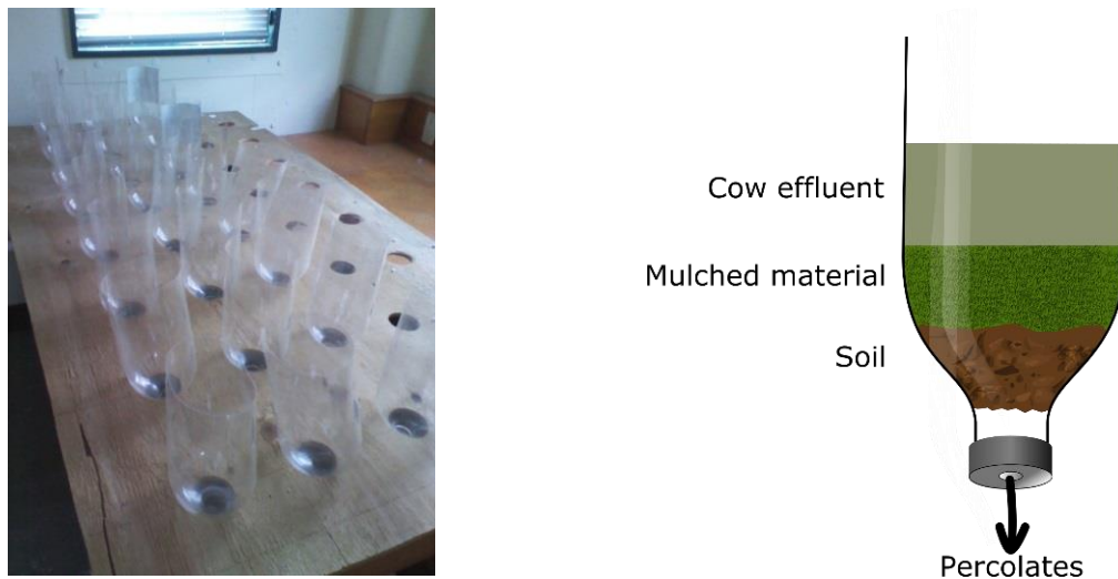
Figure 3: Laboratory lysimeter system and setup with soil, mulched material and effluent (O. Champeau)
