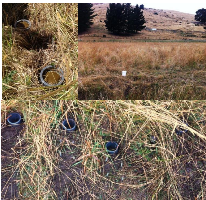
Figure 12: Lysimeters deployed at Te Kaio Farm loaded with cattle effluent (top left), lysimeters deployed along the stream (lower), and a view of the farm catchment (top right) (O. Champeau)
