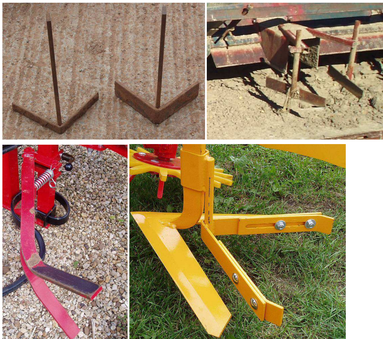
Figure 9. Various mini-ridger designs: Basic, vertical leg, V design, with two different ridger heights (top left), single blade, rotatable design on a rotary hoe / rotovator with wide crop gaps for field tomato production (top right), V design on a sloping sprung loaded leg (bottom left) and vertical leg V design with adjustable wings mounted behind a V blade hoe (bottom right).
