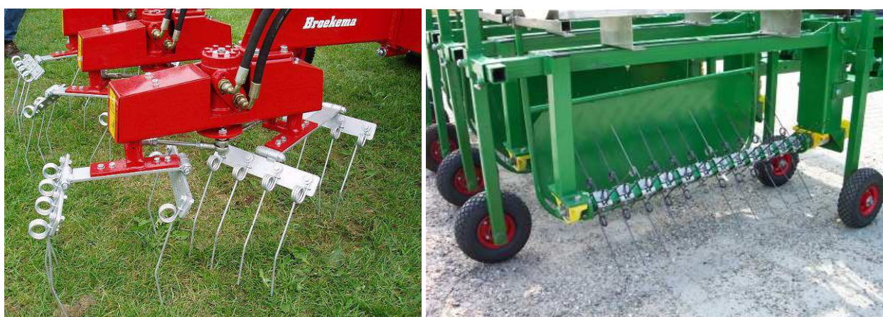
Figure 6. Vertical spring tine oscillating weeder (left) horizontal axis rotating spring tine weeder (right).
