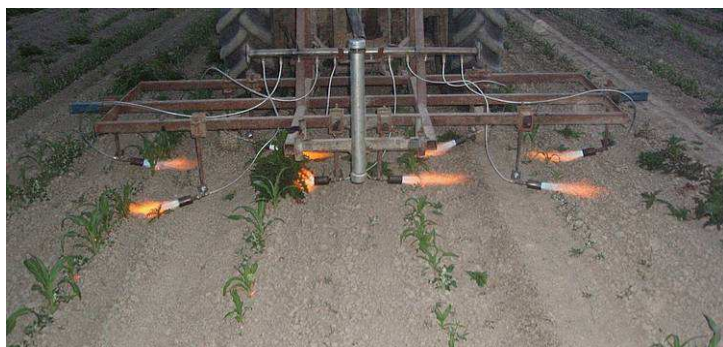
Figure 7. Non-discriminatory intrarow thermal weeder operating in sweetcorn.
