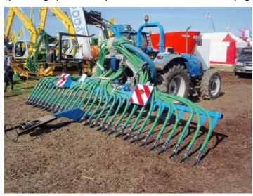
Figure 4. Umbilical system spreader
