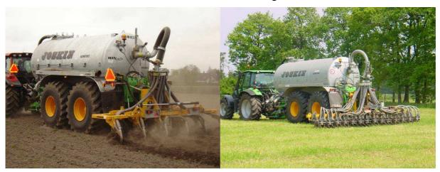
Figure 3. Equipment for injecting slurry into soil and pasture.
