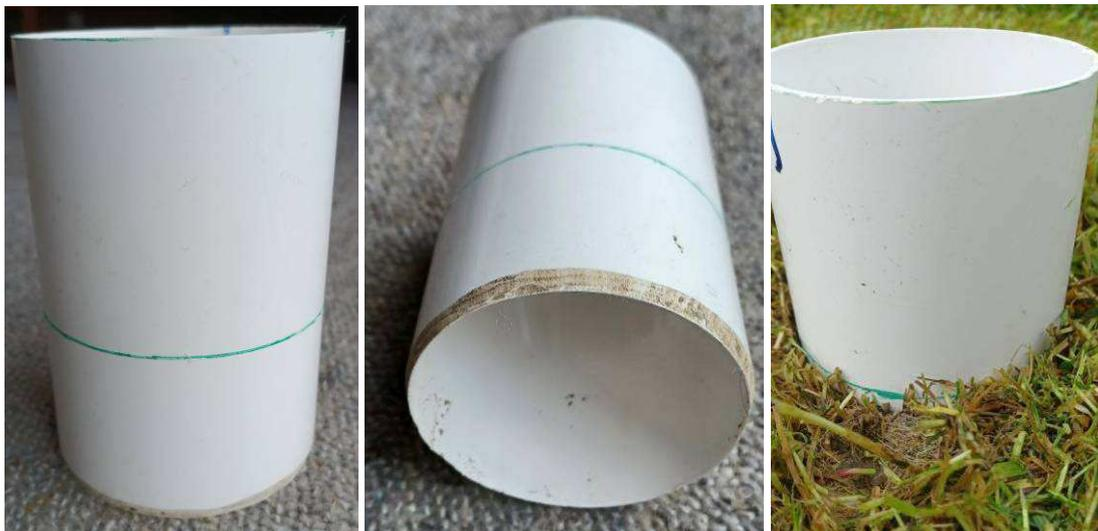
Figure 7. Ring infiltrometer made from 12 cm / 5" long, 8 cm / 3" diameter uPVC guttering down pipe, showing sharpened end for driving into soil and inserted into the soil to the depth line at 5 cm / 2".
