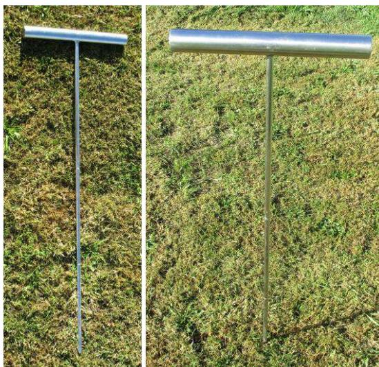
Figure 5. Soil probe.
