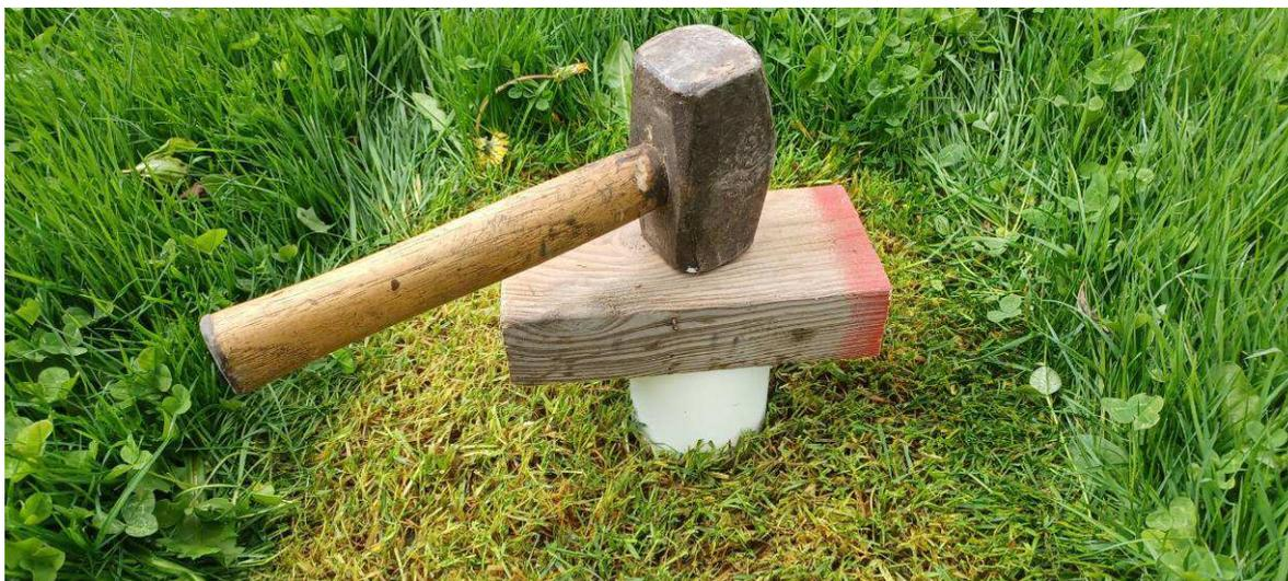
Figure 9. Simple method for driving ring into ground – wooden batten and club hammer.
