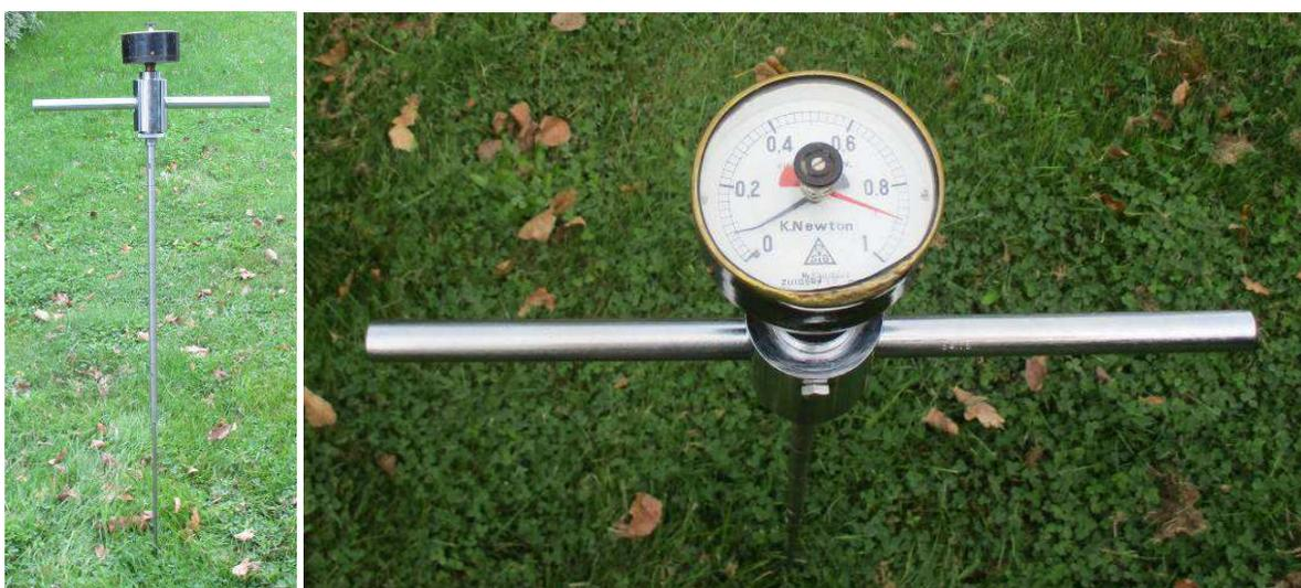
Figure 6. Soil penetrometer.
