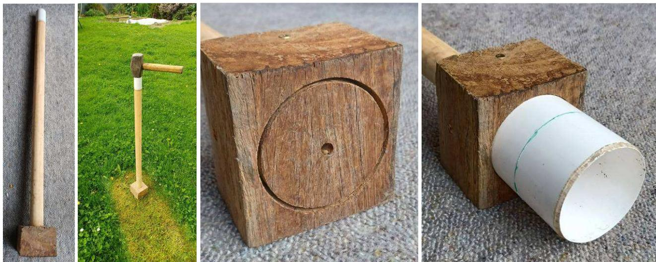
Figure 11. 'Fancy' ring driver, with a circular slot cut in a wood block with hole saw that the ring fits snugly into and with a wooden shaft to allow ring to be driven from standing position.
