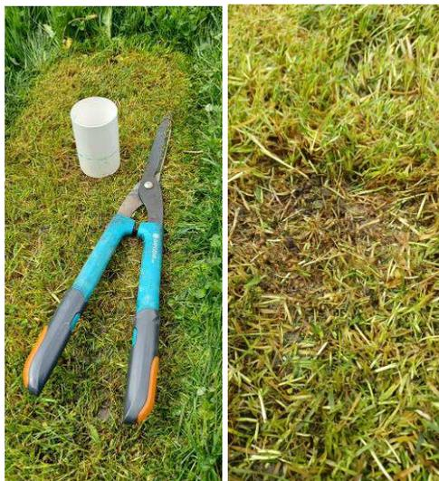
Figure 8. Ground preparation – clearing as much vegetation and residue from the test location as possible.
