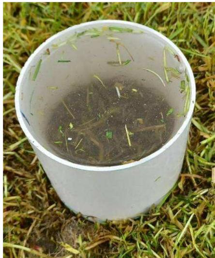
Figure 10. Infiltration ring filled with water.
