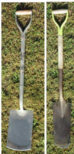
Figure 3. Standard spade left and post hole / ditching spade right.
