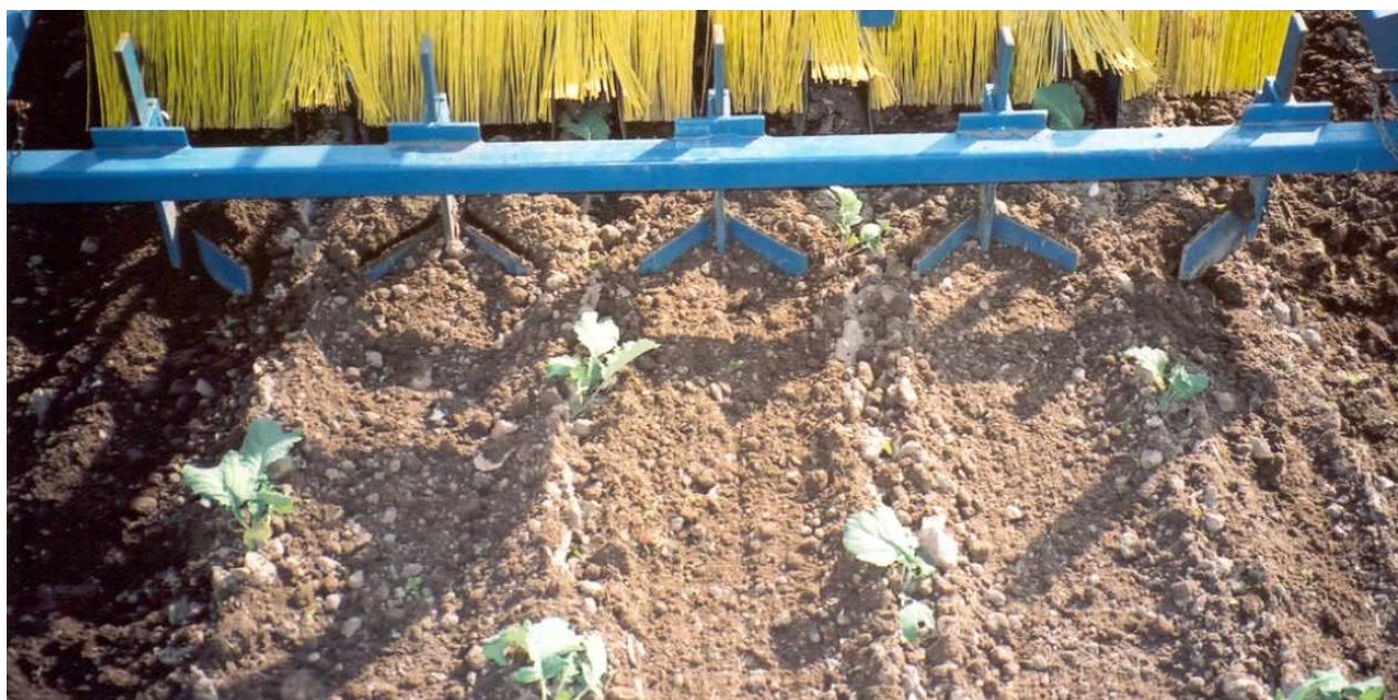
Figure 1. Mini-ridger in transplanted cabbages.
